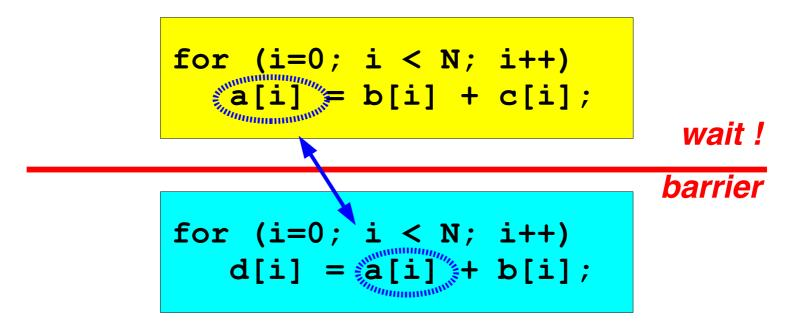
All threads wait at the barrier point and only continue when all threads have reached the barrier point
