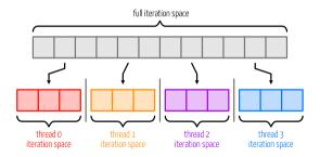
As the threads run in parallel, we can expect a nthreads speedup as each thread works on niters/nthreads iterations of the loop
