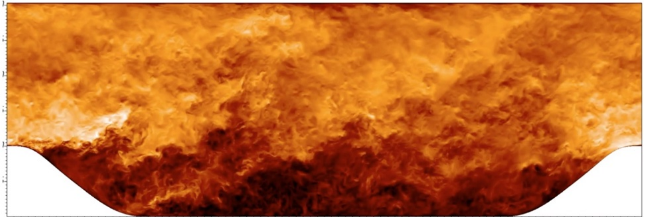
Nek5000 DNS of flow past a periodic hill at Re=19,000 on ALCF Mira. Ramesh Balakrishnan, ANL
