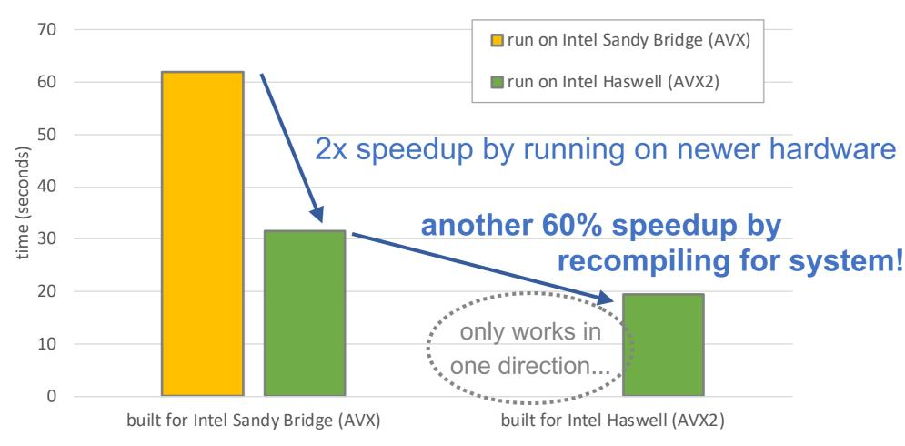
(FFTW 3.3.8 installed in Singularity container)
